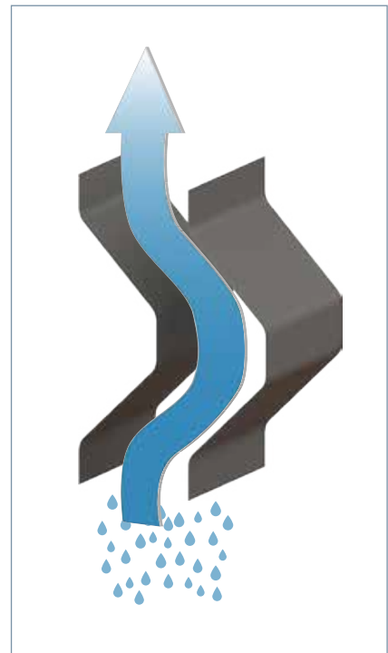
Vertical flow at the RV200 type profile
